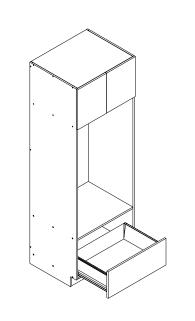
STEP 12 Put the the drawer to the carcase cabinet accessibled finished.
