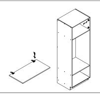
STEP 8 Press the hinges into the base, and then install doors.
